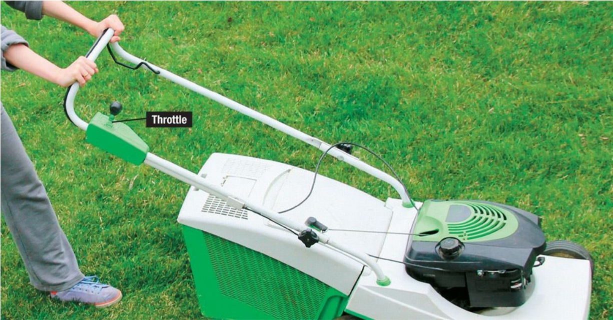
Engine speed is controlled by the throttle, a grippable lever that opens and closes the throttle plate.
